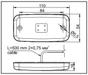
Universal amber LED side marking lamp with reflector, holding bracket and integrated cable  $2x0,75 \text{ mm}^2$ . Voltage range 12-30 V DC - non-polarised. The product is fullfilling highest quality standards. Extreme small power consumption using a 12 V cirquit 12V(0,04A)=0,5W and 24 V cirquit 24V(0,04A)=1W. Working temperature range from  $-40^{\circ}\text{C}$  to  $+100^{\circ}\text{C}$ .
